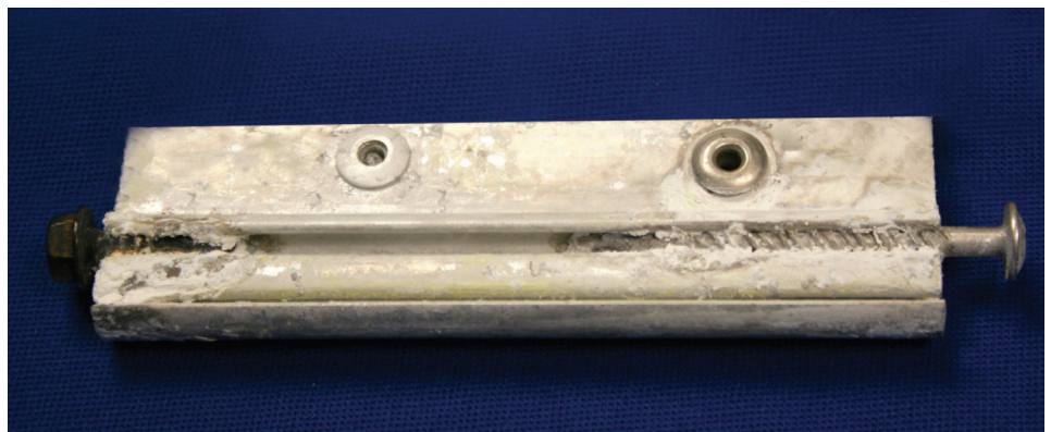
Left screw: Leading screw coating for aluminum. Right screw: 18-8 Stainless steel.
