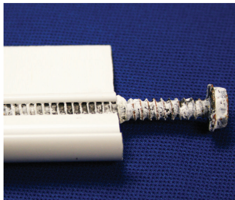
In accelerated lab tests, other coatings degrade like this.
